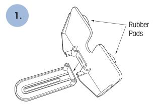
The cleats are supplied in two parts and must be clipped together and attached to the Bathboard before fitting. The rubber pads on the cleats must face outwards to make firm contact with the sides of the bath to ensure a firm fitting. This applies to both cleats.
