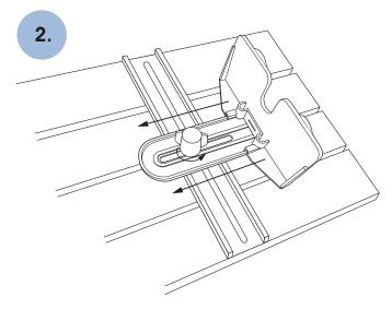
Loosen the wing screws and move the cleats towards the centre of the board for the narrowest fitting.
