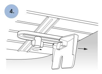
Reach under the board and push the cleats outwards until they touch the inside walls of the bath, then tighten the wingscrews.
