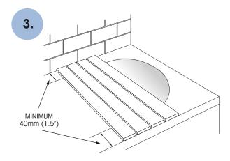
Place the board across the bath at the position where it is to be used, with the cleats on the underside. The rim of the bath must support at least  $40\text{mm} \ (1.5'')$  of the end of the board, on both sides of the bath.
