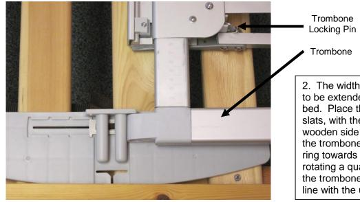
2. The width adjusting "trombone" needs to be extended to suit the width of the bed. Place the strap bracket on the slats, with the curved side touching the wooden side rail of the bed. Disengage the trombone locking pin by pulling the ring towards the head of the bed and rotating a quarter of a turn. Now extend the trombone until the inside edge is in line with the upstand of the strap bracket.
