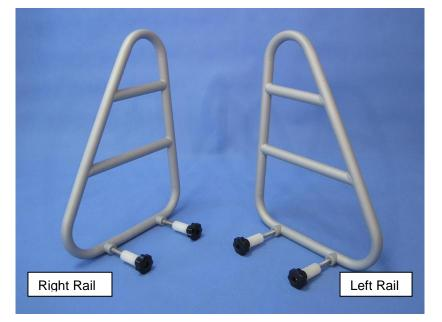
The Left and Right Side Rails are identified from the perspective of the user, lying on the bed on their back. Each rail has two threaded rods that fit through the width adjusting trombones of the DreamMaster Light, and secure with plastic spacers and hand wheels.
