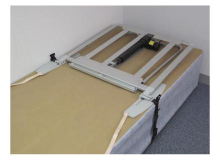
4. Connect one of the 2.5m brown straps to the lower female buckle from the strap bracket at one side of the bed. Pass the long strap under the bed and connect at the other side. Tighten the strap to secure the elevator to the bed base, then tidy away any excess strap to avoid a trip hazard.
