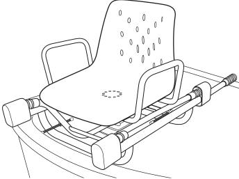
The two Positioning Screws facing in to the bath can either be adjusted so that they are out of the way, or removed. They will not perform any function.
